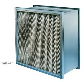
Type HT (High Temperature) Series VariCel filters are designed for systems operating from 350°-900°F. Constructed of aluminized steel, HT VariCel filters offer rated efficiency with proven reliability over the life of the filter. See page 4 for models and temperature limits. HT VariCel filters are offered in a 12" depth, MERV 14/14A and MERV 11.
