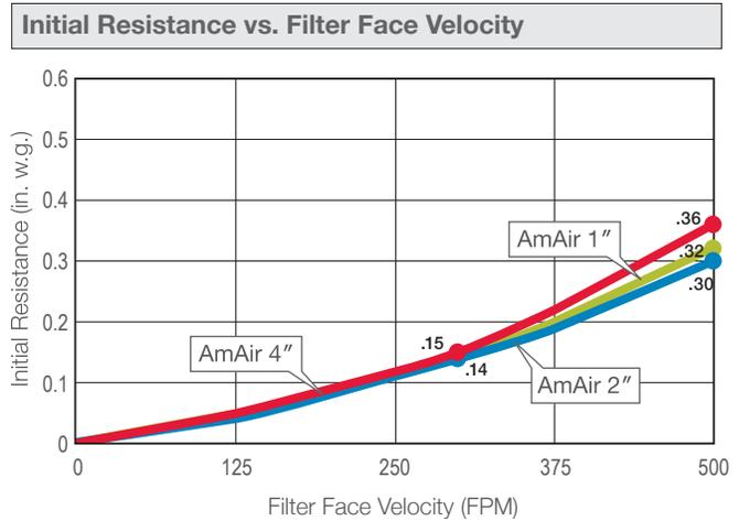
Filters are rated at 500 FPM filter face velocity. Recommended final resistance for all AmAir/CE filters is 1" w.g.
